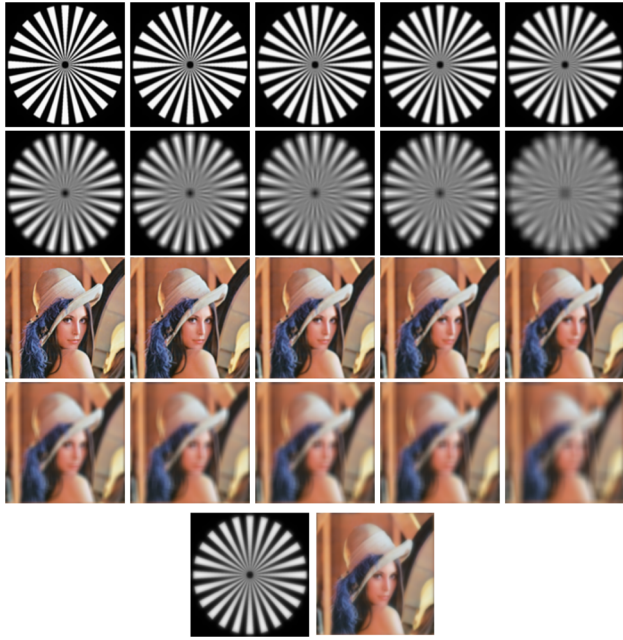
F6:1 Fig. 6. Averaging 10 snapshots having focus error coefficients F6:2 with random values.
